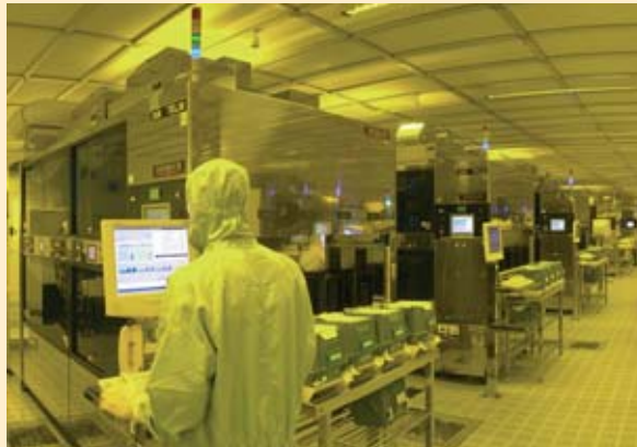
Photolithography section in ultra-clean facilities at the STMicroelectronics unit in Crolles (Isère).
