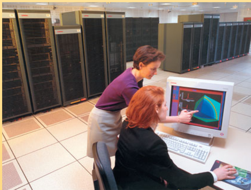
Installed at CEA (DAM-Ile de France Center) in December 2001, the TERA machine designed by Compaq (now HP) has for its basic element a mini-computer with 4 x 1-GHz processors sharing 4 GB of memory and giving a total performance of 8 Gflops. These basic elements are interconnected through a fast network designed by Quadrics Ltd. A synchronization operation across all 2,560 processors is completed in under 25 microseconds. The overall file system offers 50 terabytes of storage space for input/output with an aggregate bandwidth of 7.5 GB/s.
