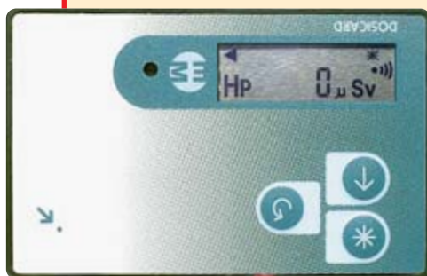
Dosicard dosimeter for real-time dosimetric monitoring.
