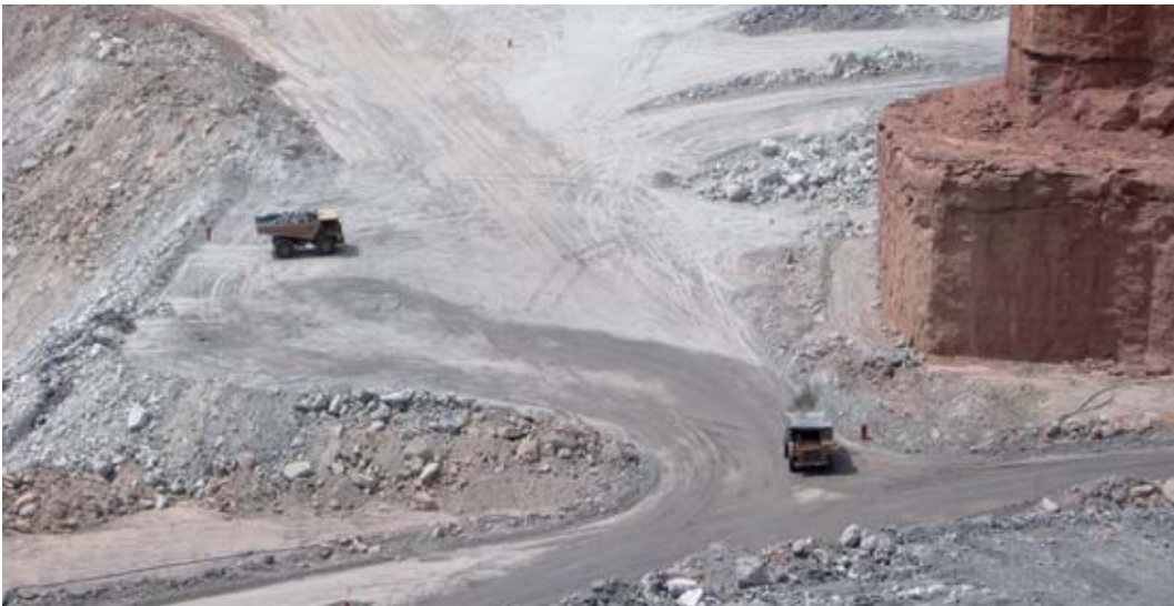
Somair open-pit mine, at Arlit (Niger). Backfill methods using the mine's own waste (tip visible below truck at left) make for better workings economics, and help limit landscape and environmental impact, however they do virtually preclude subsequent recovery of mineral-bearing areas abandoned at the bottom of the pit, or of low-grade "dead rock."
