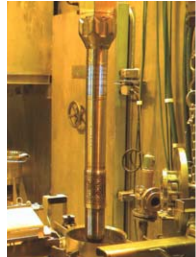
Figure 3. Foot of an irradiated Superphénix assembly, before (left), and after (right) washing. For future reactors, investigations will address improvements to washing techniques, to bring down overall campaign time.
