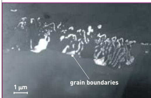
Figure 6. Precipitation of M_{23}C_6 carbides at the grain boundaries. – Alloy 617 after 1,000 h aging at 850 °C (from L. Guetaz).
