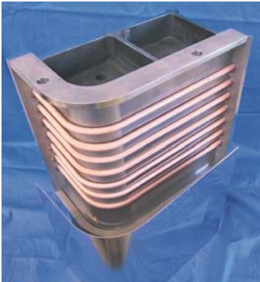
Eurofer-copper ITER TBM (test blanket module) mockup (prior to hot isostatic pressing), representative of part of a fusion reactor tritium-breeding blanket.
