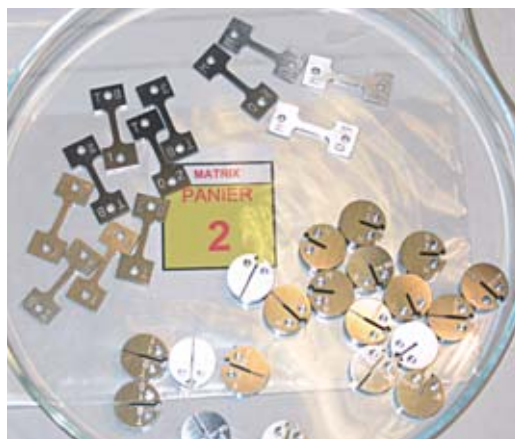
A batch of samples of materials intended for nuclear systems of the future, readied for the MATRIX experimental irradiation program, in the Phénix reactor.
