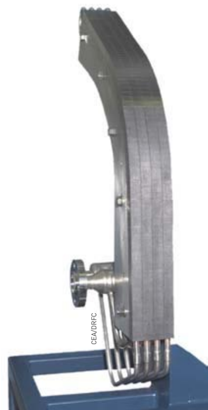
Carbon-carbon (C-C) composite used in the Tore Supra fusion machine, for the first (inner) wall, facing the plasma (the component is 1 m long).
