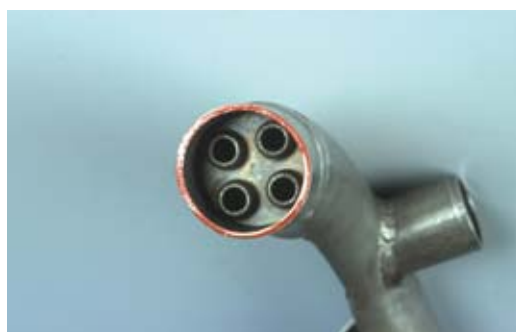
H-meter, for the detection of hydrogen. The hydrogen that may be contained in the sodium circulating along the four nickel tubes diffuses across that metal, arriving in the space under vacuum surrounding the tubes, where a spectrometer measures concentration of the gas.
