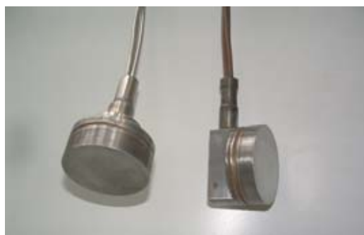
Two types of high-temperature ultrasonic transducers (TUSHTs).
