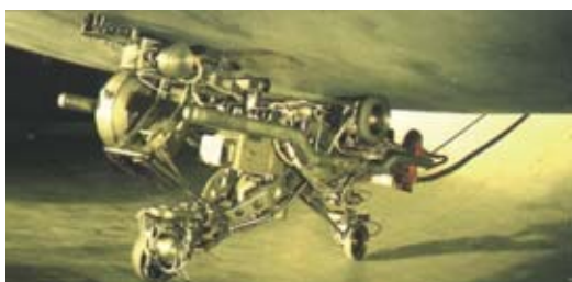
The MIR inspection robot, used to test main vessel welds in the Superphénix reactor, seen here in the space extending between that vessel and the safety vessel.
