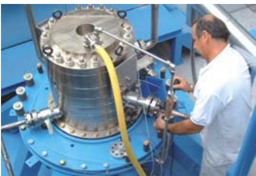
A compressor, featuring peripheral stages and a rotating assembly operating in gas, being readied for tests.
