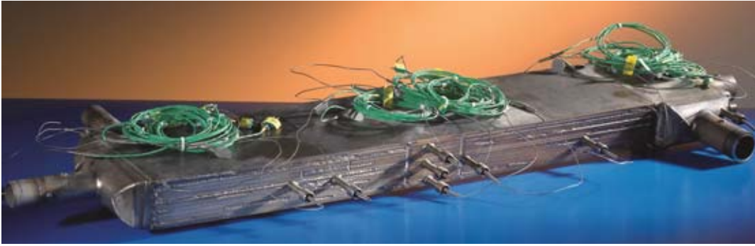
Mockup of a Nordon-technology heat exchanger for a very-high-temperature reactor, as tested on the CLAIRE loop, at Cadarache. The thermocouples may be seen (in green).
