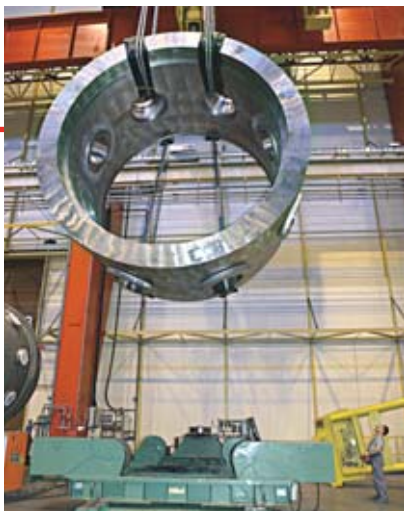
Pressure-vessel nozzle shell for EDF's Flammanville 3 reactor, the first EPR to be built on French soil.
