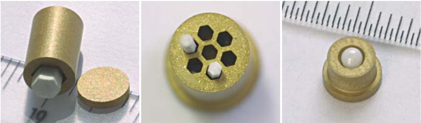
Innovative GFR fuel concepts, investigated in the FUTURIX-Concepts experiment.
