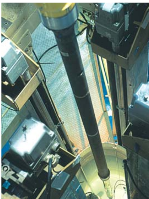
Positioning a fission chamber in the MINERVE reactor driver core.
