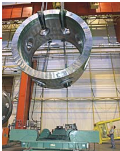
Pressure-vessel nozzle shell for EDF's Flamanville 3 reactor, the first EPR to be built on French soil.
