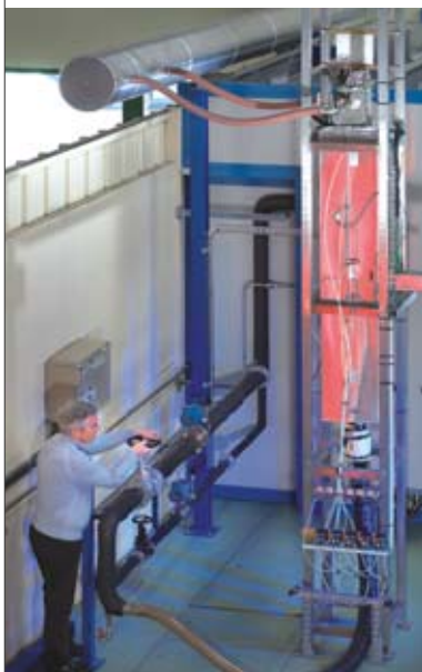
The ESTHAIR (Essais thermoaérodynamiques en air: Gas Thermal-Hydraulic Tests in Air) facility, at CEA's Grenoble Center, intended, in particular, for the evaluation of friction and heat exchange coefficients for the pin-type fuel element for the ETDR startup core.
