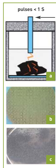
Figure 2. Principle schematic of breakup by pulsed currents yielded by a Marx generator, with a voltage in the 200–500 kV range, and intensity of 10–20 kA (a), and view of an SiC honeycomb structure with cells filled with SiC (dispersed fuel), before pulsed-current treatment (b), and after 30 pulses (c).
