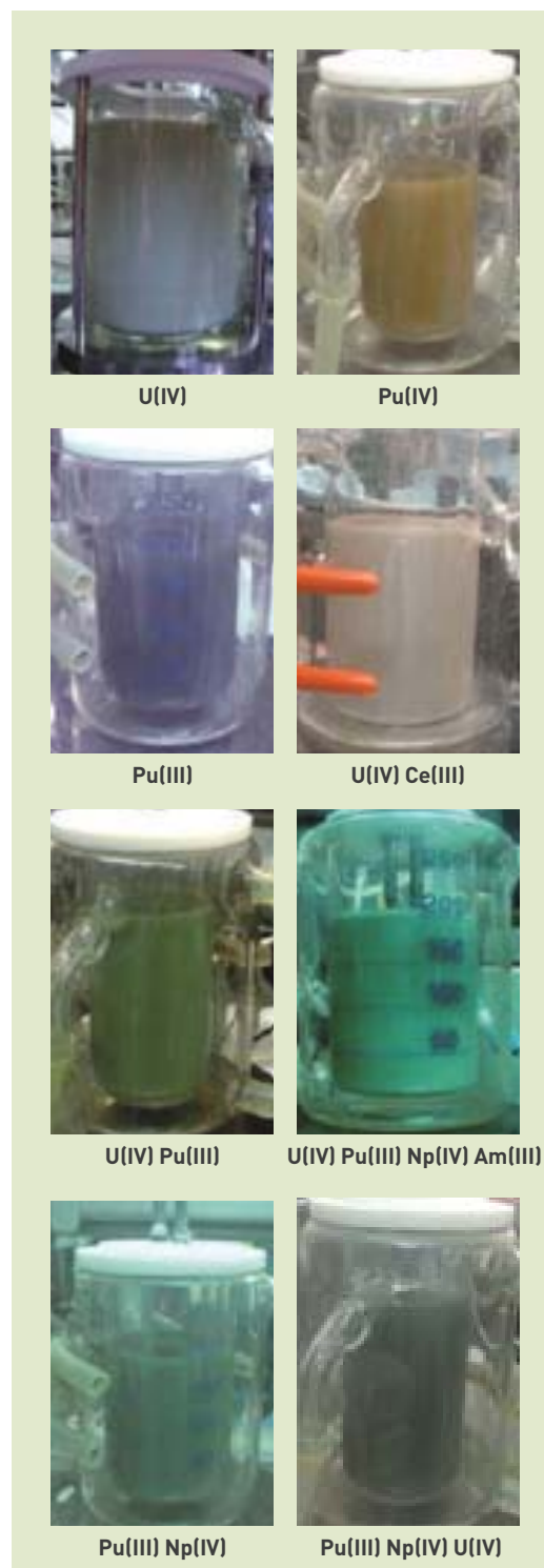
Figure 7. Co-conversion tests with actinides at various degrees of oxidation, carried out in ATALANTE.
