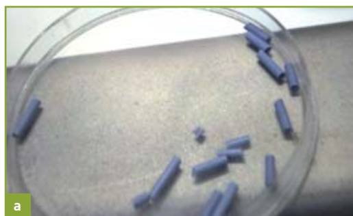
Figure 8. a) The salt seen before contact [blue color, characteristic of Pu(III)]. b) Salt after contact (brown color, characteristic of lanthanides), after extraction of the actinides.
