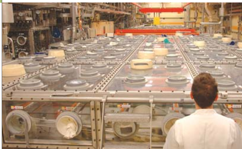
Gloveboxes used for the cladding of MOX fuel rods, in the Melox plant, at Bagnols-sur-Cèze (Gard département, southern France).
