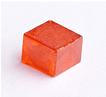
Perovskite single crystal grown in solution © Dominique GUILLAUDIN/CEA
