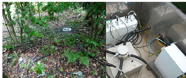
Image showing an infrasound station and a microbarometer used to measure variations in atmospheric pressure. © CEA-DAM
