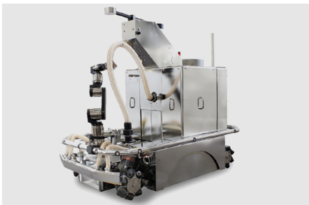
Gobie, a remote control device for clean-up of working areas. © CEA
