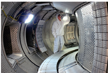
Inside the tokamak: on the left are two antennas for ICRH heating on the outside walls. The two heating systems can heat plasma by induction. © C.Roux/CEA
