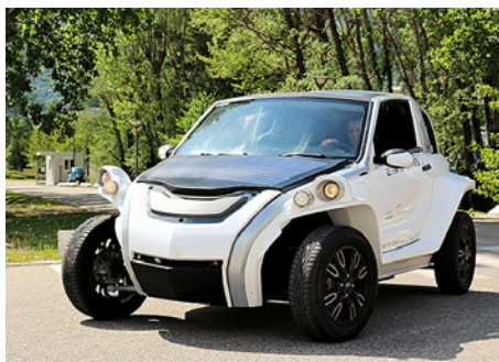
Solar car project fitted with solar panels in its bodywork. © CEA
