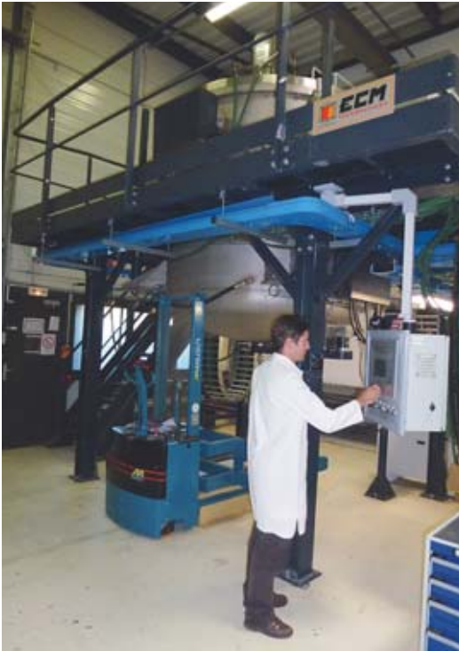
Silicon crystallization oven. The silicon is heated to its melting point. As it cools, the molten silicon solidifies, forming a single, large crystal (monocrystalline silicon) or several crystals (polycrystalline silicon). The silicon ingots are cut into very fine wafers (about 200 microns thick) used to create the photovoltaic cells.
