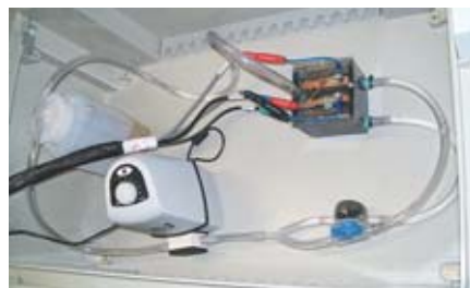
Prototype of a honeycomb flow-through electrodes reactor (left) from which a prototype Pb-MSA redox flow battery was built (right). Visible are the electrolyte tank, the pump (white), the reactor and the electrolyte circulation indicators (blue and black).
