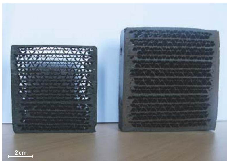
Flow-through electrode before calcination (right, composite of phenolic resin and cellulose) and after calcination (left, vitreous carbon, low-density carbonaceous material).
