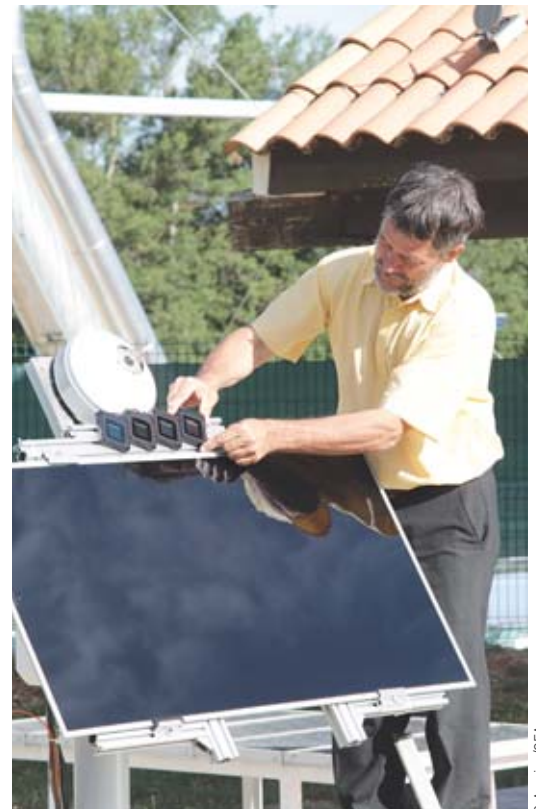
Thin film photovoltaic module. In addition to its significant involvement in the silicon sector, CEA is conducting numerous studies into thin film technology.
