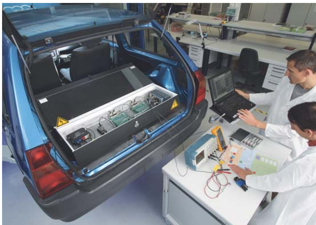
Development and validation of the battery pack management system for the CEA demonstration vehicle. This vehicle was developed from an electric Citroën AX dating from the 1990s, which at the time was the lightest electric vehicle available.
