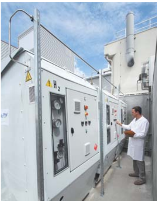
Three McPhy Energy technology hydrogen storage tanks being tested at the Liten Institute/DTBH. These tanks store hydrogen in a magnesium hydride (MgH 2 ). Their particularity lies in the fact that the hydriding heat is stored in a phase change material and then restored at desorption. They can each store 5 kg of hydrogen at the maximum pressure of 10 bar.
