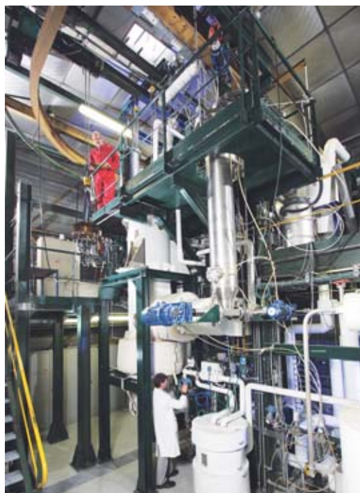
High Temperature Fluidized Bed (HTFB), for the production of synthesis gas from biomass, located in the CEA Grenoble Center. An input of nuclear heat would help with gasification without consuming hydrocarbons.
