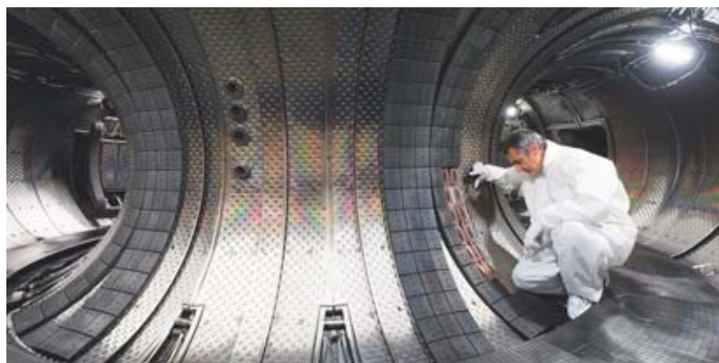
The vacuum chamber of the Tore Supra tokamak. Tore Supra was installed in the CEA Cadarache Center and entered service in 1988. It is mainly devoted to studying the physics and the technologies needed to produce long-duration high-performance plasmas. It is the only European tokamak to combine superconducting components and actively cooled plasma facing components. It led to major scientific and technological advances for ITER.
