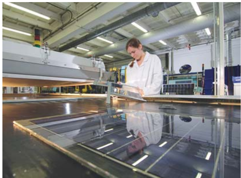
Lamination, one of the manufacturing steps of photovoltaic modules. This operation consists in heating the modules (photovoltaic cells and encapsulating materials) while pressing them in a partial vacuum to eliminate any residual gases.
