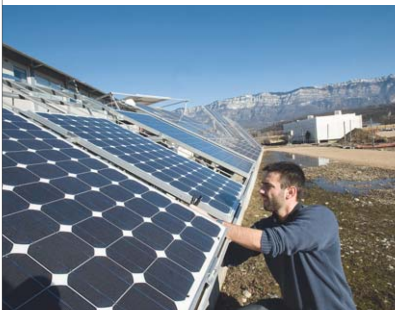
Comparative test bench for the various photovoltaic technologies. The modules are being installed.
