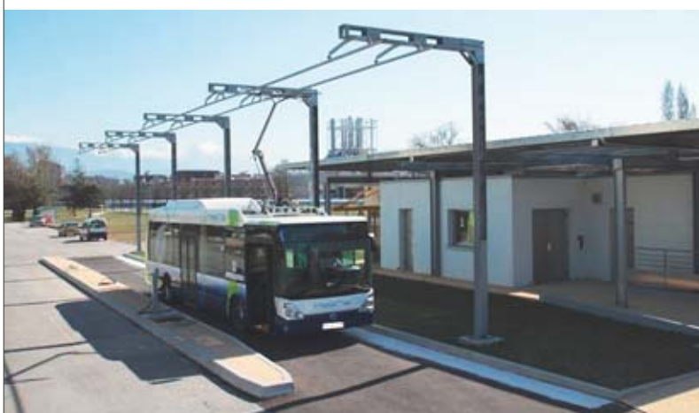
Recharging an Irisbus rechargeable hybrid bus at the CEA Grenoble fast recharge station.
