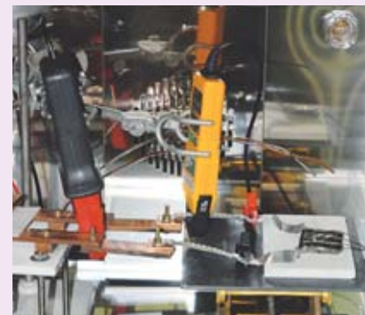
Electrical short-circuit test. The short-circuit is created by connecting the positive and negative poles of a cell by means of a metal conductor with negligible resistance. This test simulates an external short-circuit.
