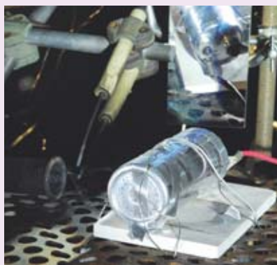
Thermal test: fire caused by heating with a blowtorch. This experiment consists in overheating a cell with a blowtorch, in observing its behavior over time and in testing the usual extinguishing means (water, CO 2 , etc.).
